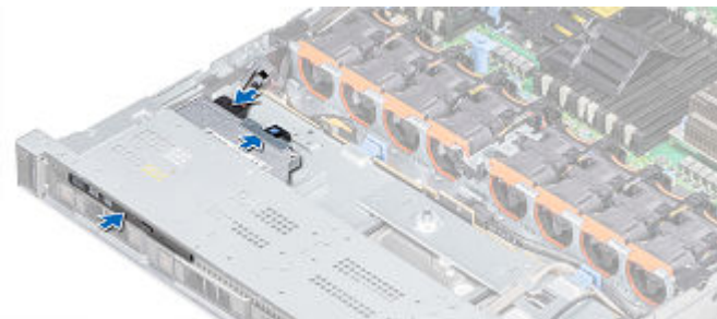
Figure 47: Optical drive insertion
