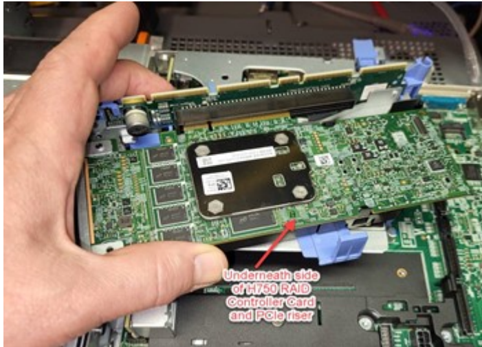
Figure 43: Turn over the expansion riser, open the blue card retainers and remove the bad H750 RAID controller
