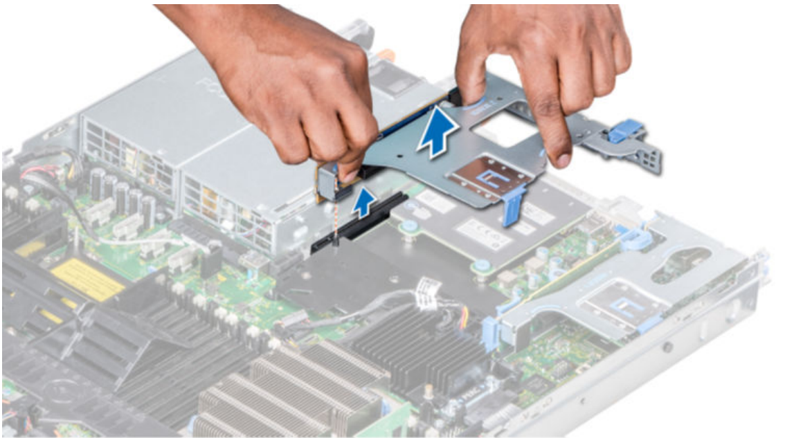
Figure 34: Remove expansion riser 2B (2 CPU systems with H750 RAID controller)
