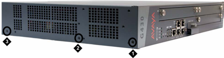
Figure 18: Removing G430 cover screws from the left side
