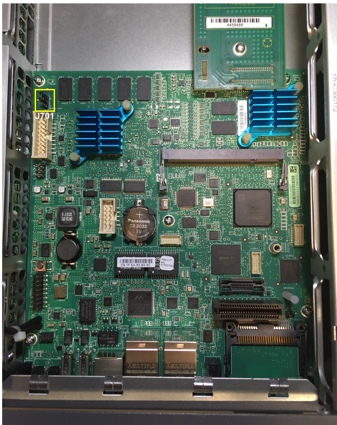
Figure 23: Branch Gateway G430 v3 NVRAM INIT J701 Jumper Location
