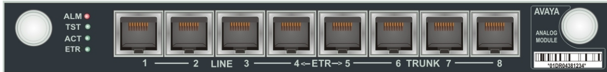
Figure 30: The MM714B media module front panel
