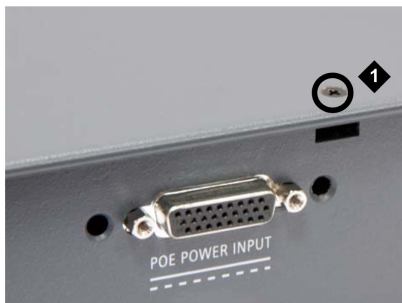
Figure 16: Removing the G430 cover screw from the top of the device
