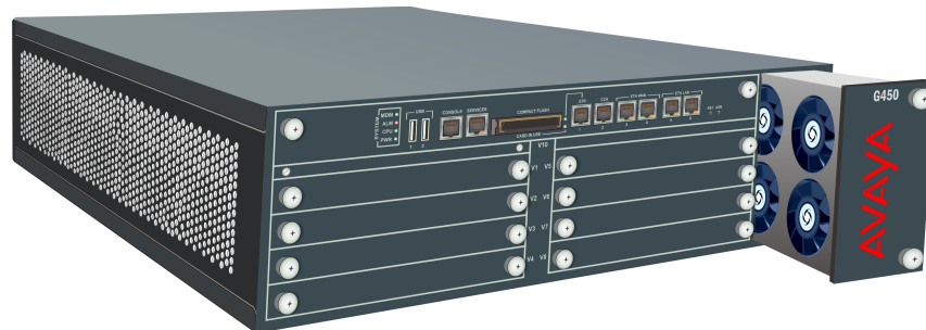
Figure 25: Replacing the fan tray
